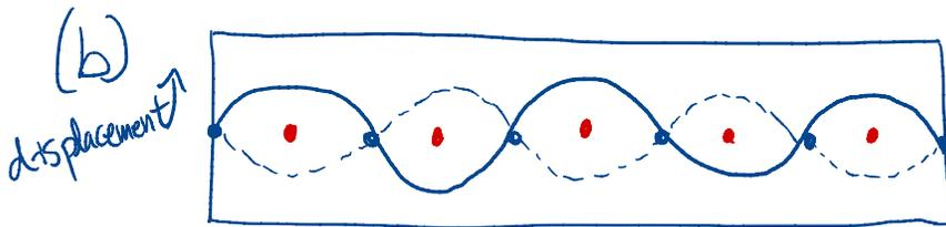
(c) The human ear responds to the applied force of a sound wave, or the pressure variations, so at the pressure nodes/displacement antinodes, one hears nothing.
