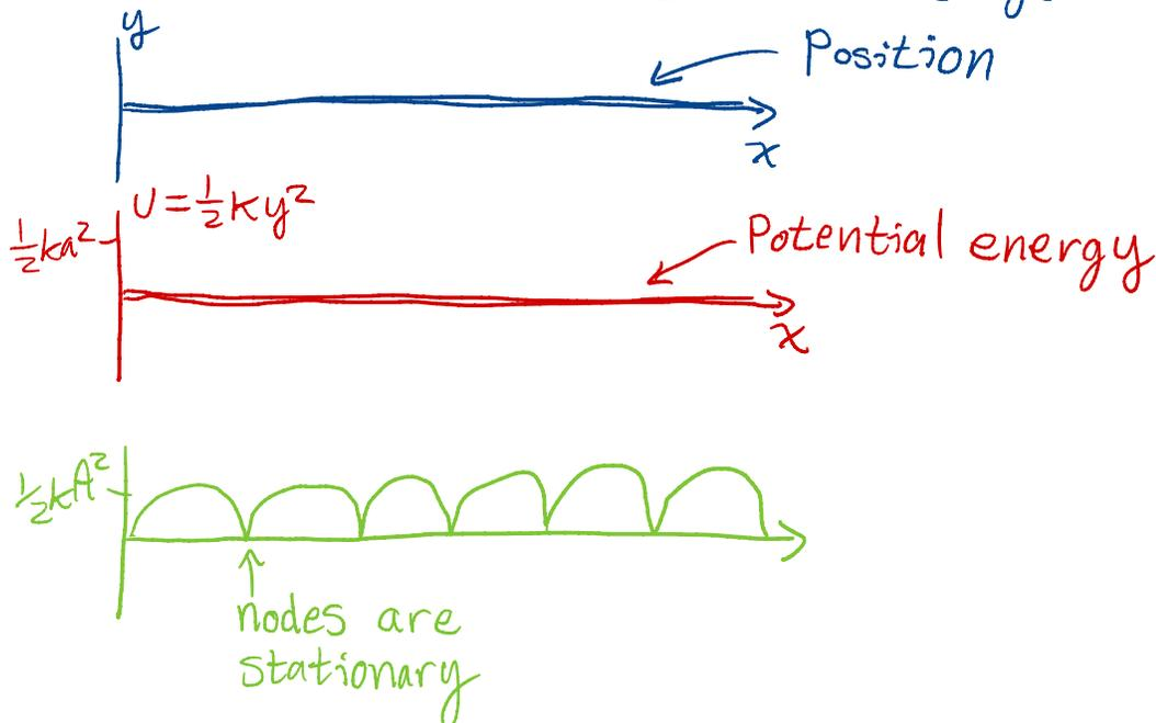
observation: the energy per unit length is constant for the traveling wave and variable for the standing wave
