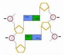
Assuming that ribose acts as a dielectric with dielectric constant 60, and the separation of the positive and negative charges is  $10^{-9}$  [m], find the voltage difference between a phosphate and an nucleotide. Note that the charge of an electron is  $1.6 \times 10^{-19}$  [C]. (4 points)
